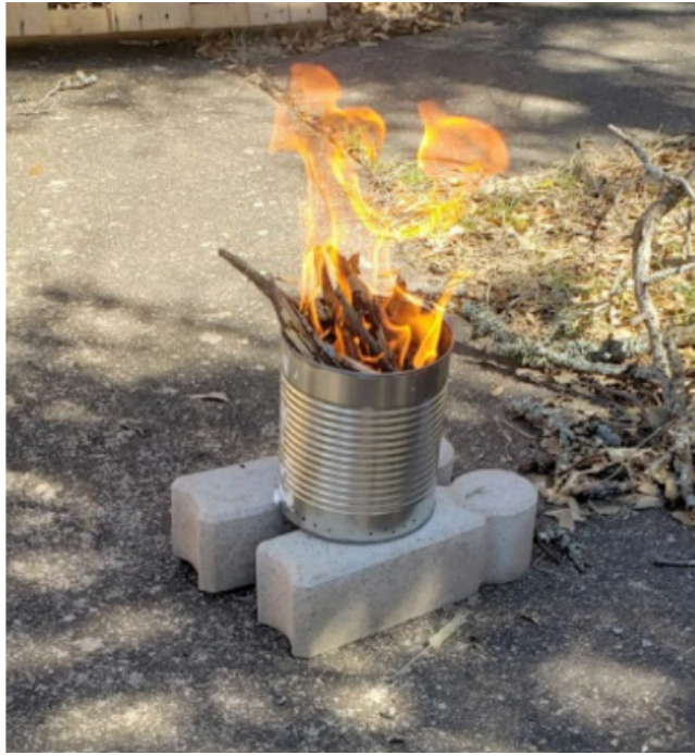
Figure 1. Early metal can kiln setup with airflow holes at the bottom.
