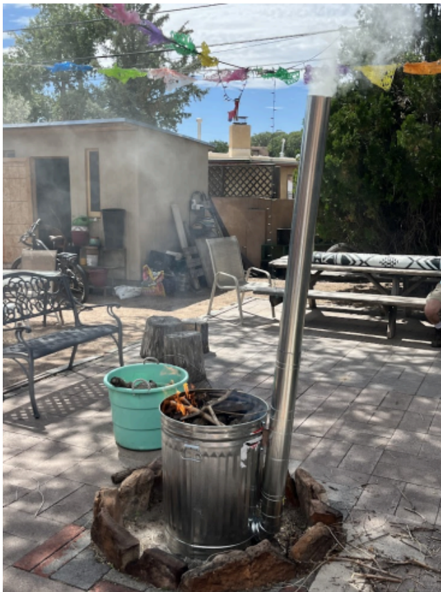
Figure 2. Downdraft bucket kiln inspired by Randy Brodnax, built by Luis Orozco, Samia van Hattum, and Fabiola De la Cueva at Samia's house. Picture courtesy of Samia van Hattum.
