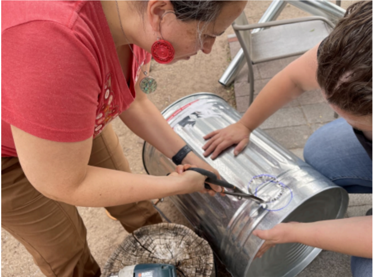
Figure 3. Drilling and cutting the intake hole at the base of the trash can.
